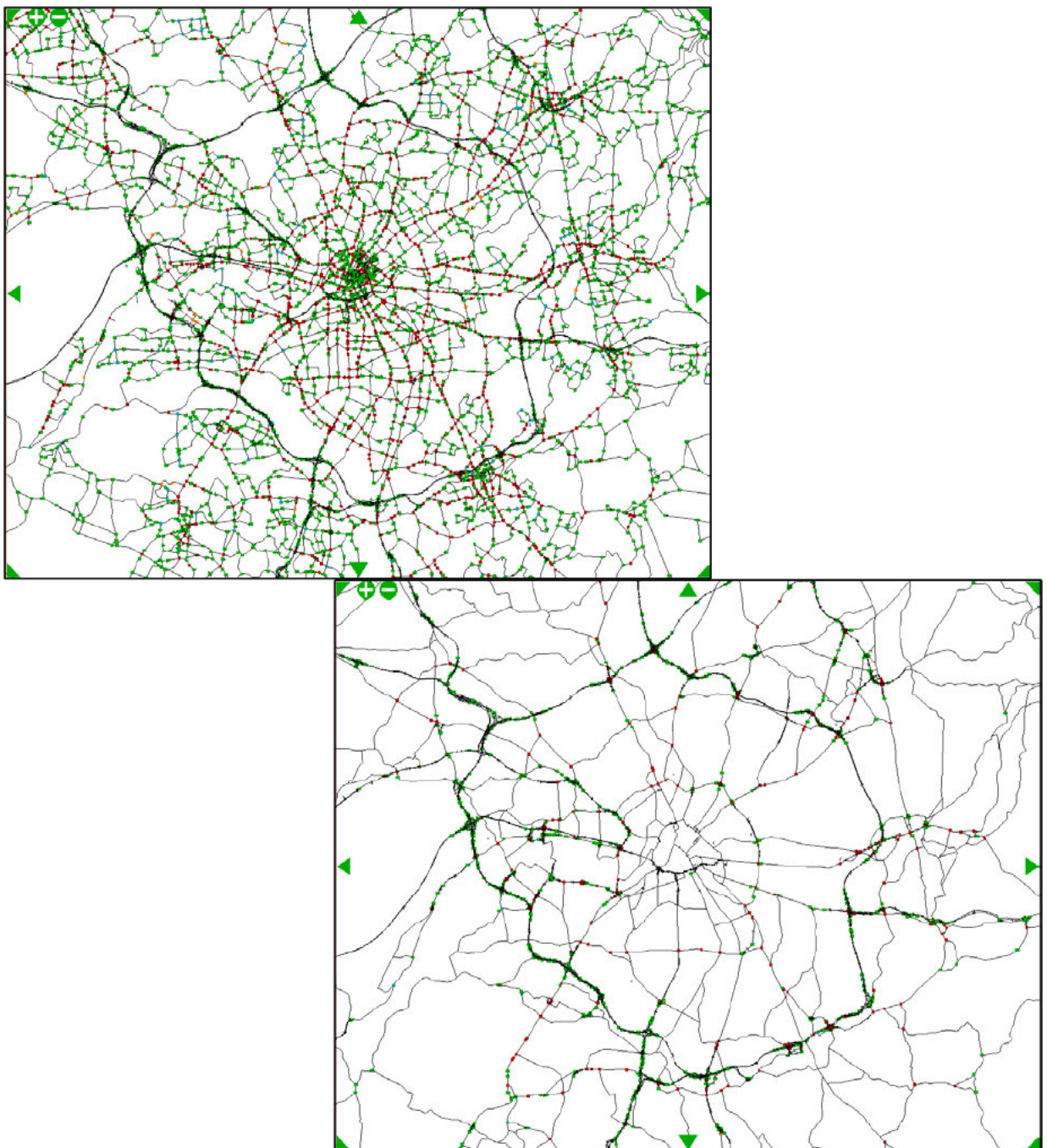
Figure 2 Simulation Network Coding – GM Model (top) vs. TPS Model (bottom)
