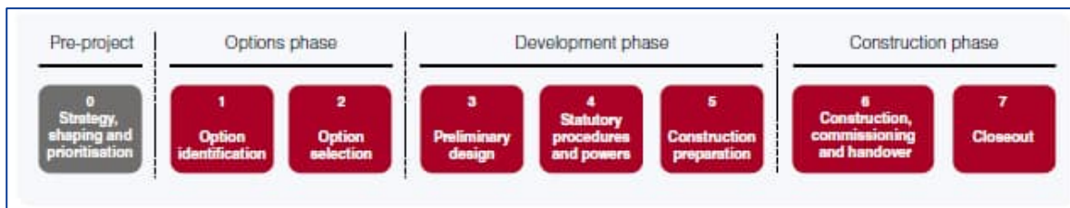
Figure 1-2 Project Control Framework
